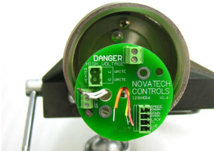
3.12 Lift the circuit board over the heater, O 2 +ve, T/C +ve and T/C -ve wires.
